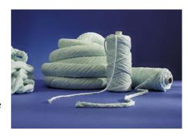
**Ecomab® Twisted Rope** is reinforced with glass (650°C) or metal wire (1050°C) and contains approximately 20% organic carrier fibre to facilitate the carding process. The carrier fibre burns out at a low temperature, but this has no effect on the properties of the speciality glass fibre.
