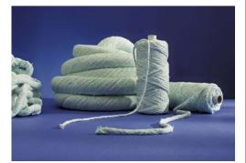
Ecomab<sup>®</sup> Twisted Rope is reinforced with glass or metal wire and contains approximately 20% organic carrier fibre to facilitate the carding process. The carrier fibre burns out at a low temperature, but this has no effect on the properties of the speciality glass fibre.
